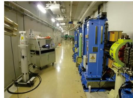
Figure 3: Leica SMART310 laser tracker.
