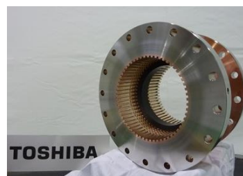
Figure 8: Prototype HOM absorber.
