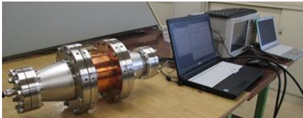
Figure 10: Set up for RF test of the prototype HOM absorber at room temperature.
