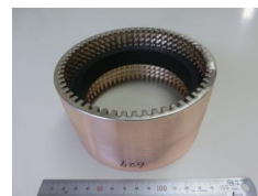
Figure 1: Test piece of brazing.
