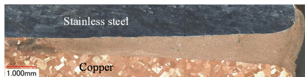
Figure 5: Micro structure of the welding cross-section.
