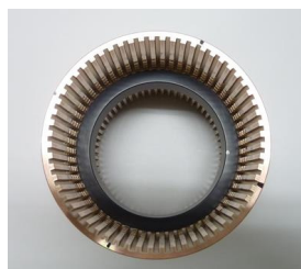
Figure 7: AlN/Cu cylinder after brazing.
