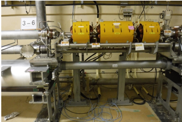
Figure 4: Photograph of the existing DC quadrupole triplet.
