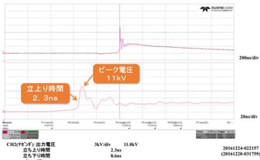
Figure 8: A waveform of an output voltage in SOS type pulse generator using SiS-DSRD.
