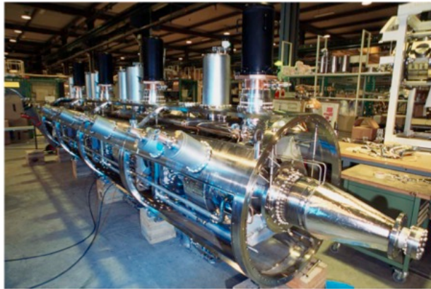
Main 400MHz RF Accelerating System (Four-Cavity Cryomodule)
