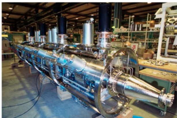
Main 400MHz RF Accelerating System (Four-Cavity Cryomodule)
