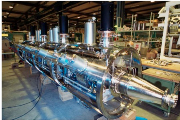
Main 400MHz RF Accelerating System (Four-Cavity Cryomodule)
