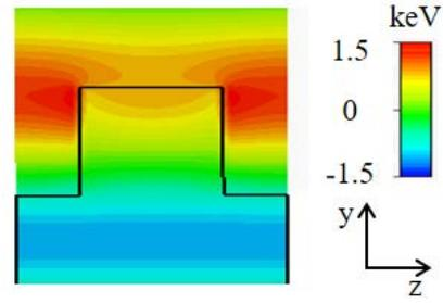
Figure 3: Distribution of the longitudinal electric field normalized to the incident laser electric field in the YZ plane.
