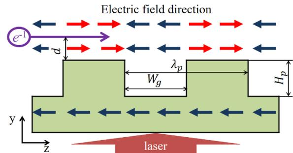
Figure 1: Principle of the single grating accelerator.
