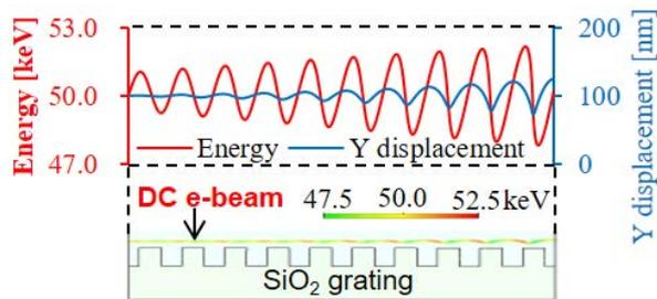
Figure 6: The PIC simulation results for a DC electron beam (colourful curve: snapshot of energy and position of electrons, red: energy, blue: Y displacement).
