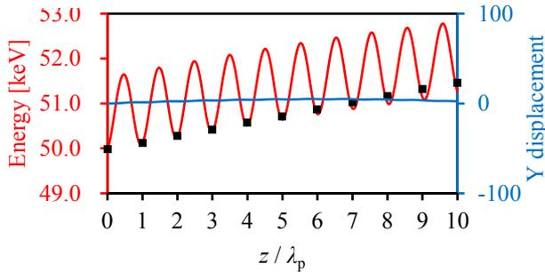
Figure 5: The comparison of PIC simulation results (red: energy, blue: displacement in Y direction) for an electron injected at the optimum accelerating phase with field simulation results (black dots: energy of electron predicted by  $G_{acc} = 0.035E_0$ ).
