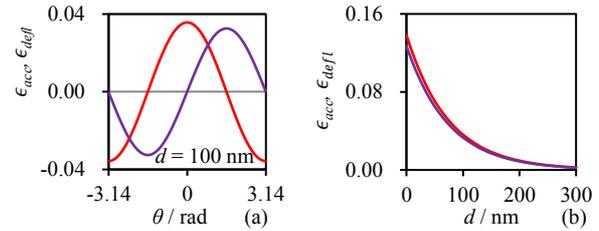
Figure 4: The amplitude of normalized acceleration gradient (red) and deflection gradient (purple) as a function of start phase  $\theta$  (a) and electron-grating distance  $d$ .
