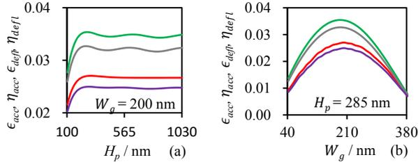
Figure 2: The amplitude of normalized acceleration gradient  $\epsilon_{acc}$  (green), acceleration factor  $\eta_{acc}$  (red), normalized deflection gradient  $\epsilon_{defl}$  (grey) and deflection factor  $\eta_{defl}$  (purple) as a function of the pillar height (a), and the groove width (b).
