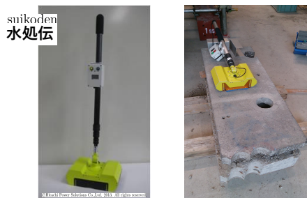
Figure 5: Moisture detection experiment using neutron moisture gauge.
