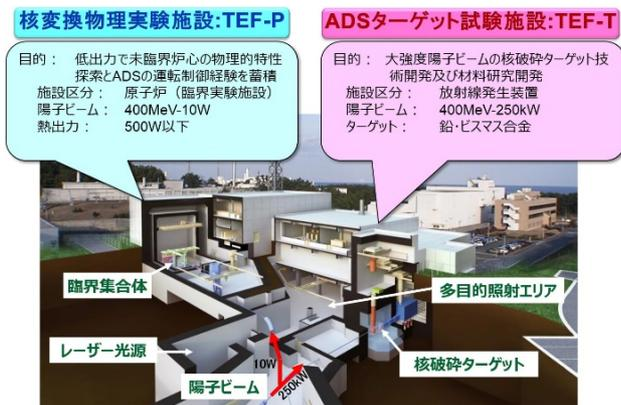
Figure 1: Transmutation Experimental Facility.
