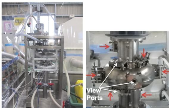
Figure 2: Photo of VEP setup(left) and coupon cavity(right).
