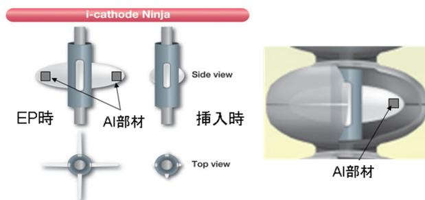
Figure 1: Schematic view of new Ninja cathode with partial metal wings.
