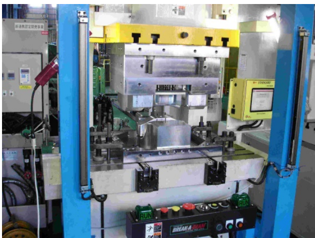
Figure 2: Assembled die set was mounted to press machine.
