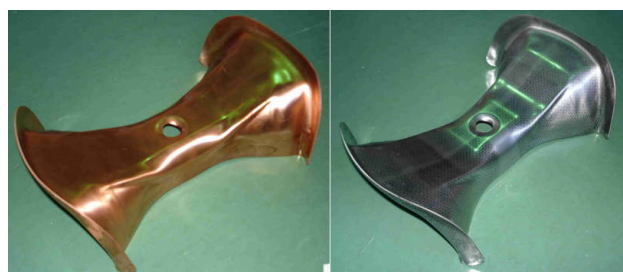
Figure 3: Press forming of half-spoke with 1.5 mm thick plates of copper (left) and aluminum (right).
