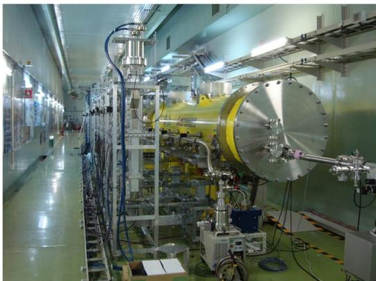
Figure 1: STF2 cryomodules.
