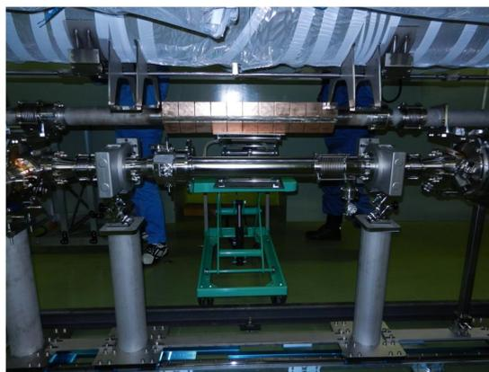
Figure 12: String assembly of CM1 in STF tunnel.
