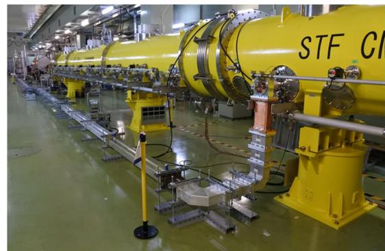
Figure 2: Waveguide system for high power RF tests.
