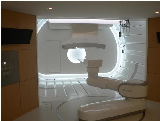
Figure 7: Photograph of covered nozzle and treatment room for rotating gantry.
