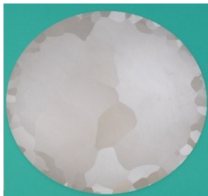
Figure1: Sliced LG Nb. The circular diameter is about 290mm.
