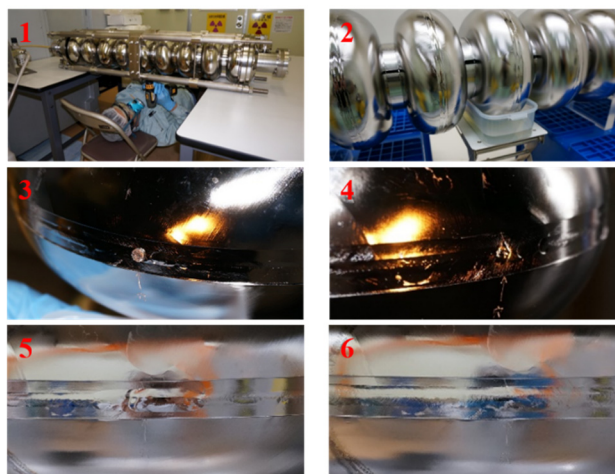
Figure 5: Repairing steps of the hole. Each numbers correspond to ones in context.
