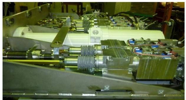
Figure 5: Picture of moving system for Deflector.
