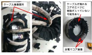
Figure 6: The balun was broken by the discharge inside.
