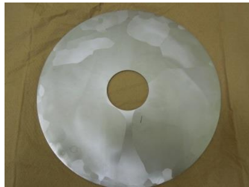
Figure 3 : Large grain Nb plate.
