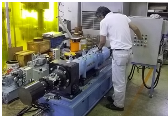
Figure 3: Hydroforming machine (Final hydraulic pressure: 25 MPa).
