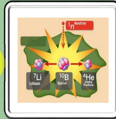
Emitted alpha particles and lithium particles destroy cancer cells
