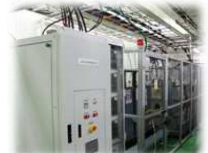
**OIST-BNCT Klystron system: 6 beams, 600 kW, -31kV, 33A**
