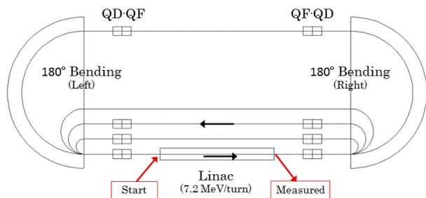
Figure 1: Components layout used in the Parmela simulation, keeping the left-right symmetry.
