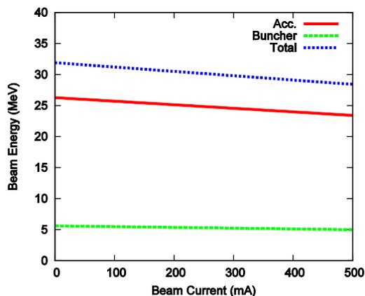
Figure 4: Relationship between beam current and beam energy.
