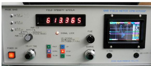
Figure 12: Measured NMR signal at the flat top of the pulsed magnetic field, with an auto-search mode.
