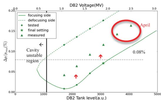
Figure 3: Simulation for DB2 amplitude tuning with simultaneous deceleration by  $0.52\text{MeV}$ , together with measurement results in Jan. and April for the focusing side.
