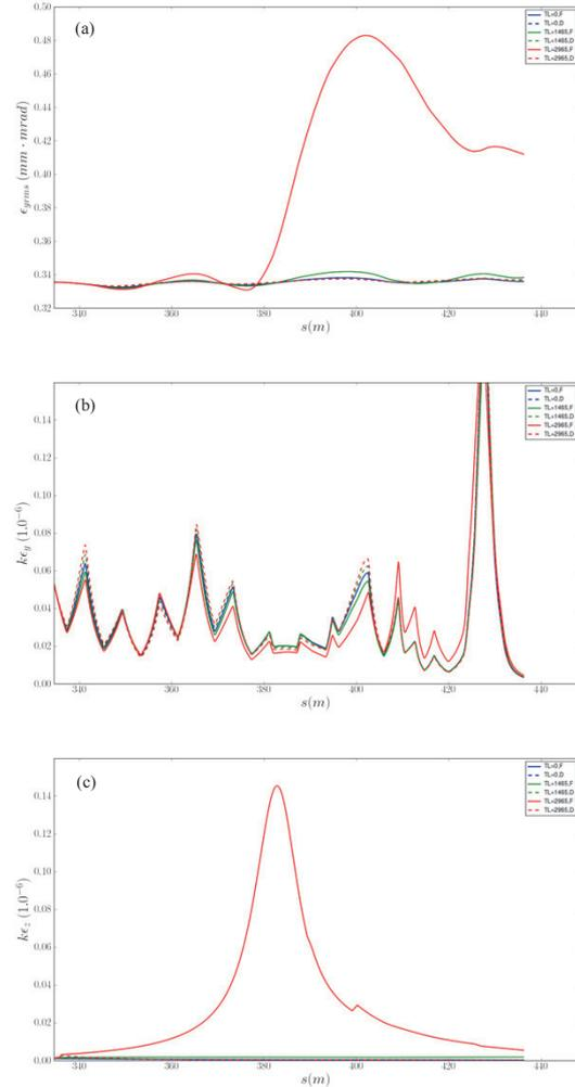
Figure 8: Simulation for experimental tested points for DB2 amplitude tuning with DB1 deceleration. (a) vertical emittance; (b) vertical “setting temperature”; (c) longitudinal “setting temperature”.
