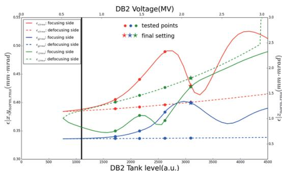
Figure 4: Simulated emittance for DB2 amplitude tuning with simultaneous deceleration by  $0.52\text{MeV}$ .
