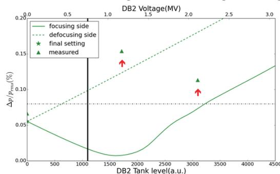
Figure 5: Simulation for DB2 amplitude tuning with DB1 deceleration, together with measurement results in June.
