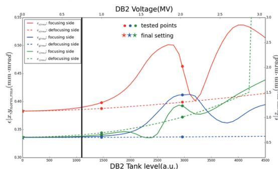
Figure 6: Simulated emittance for DB2 amplitude tuning with DB1 deceleration.
