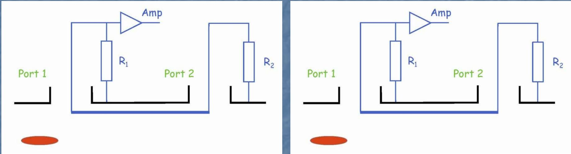
$Z_{\text{strip}} = R_1 = R_2 = 50\Omega$
