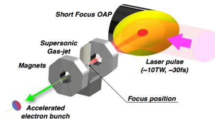
Figure 3: Experimental set up for LWFA injector.
