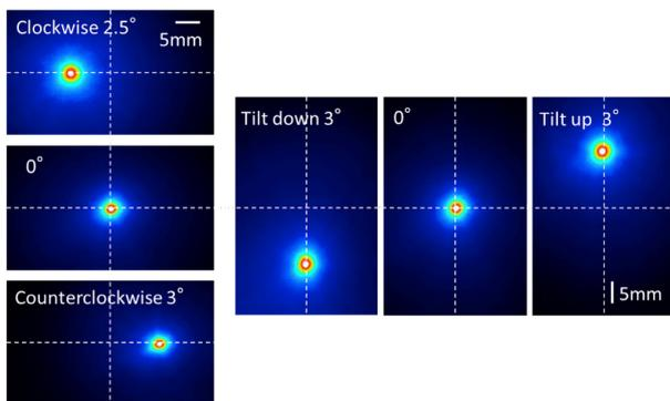
Figure 6: Pointing control of electron beams by PMO.
