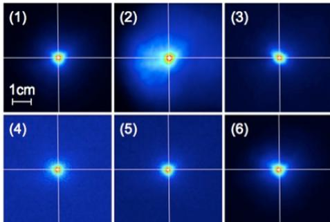
Figure 5: Electron beam profiles of 6 successive shots.
