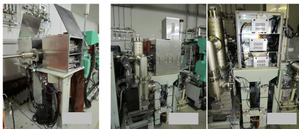
Figure 5: Counter kick systems installed in SPring-8.
