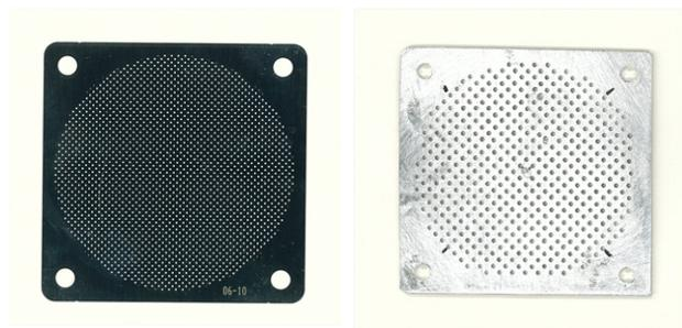
Figure 4: Left: 1/10 attenuator(each distance of hole is 1mm), right: mask(each distance of hole is 2mm).
