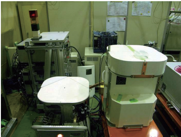
Figure 4: Photo of 950 keV X-ray source based on X-band Linac.
