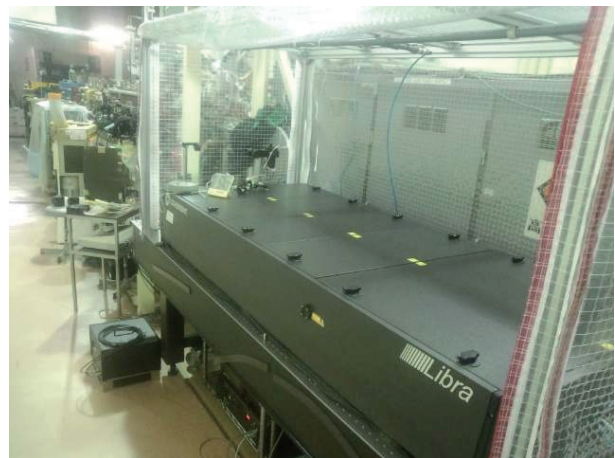
Figure 1: Photo of driving laser for S-band photocathode RF-gun.
