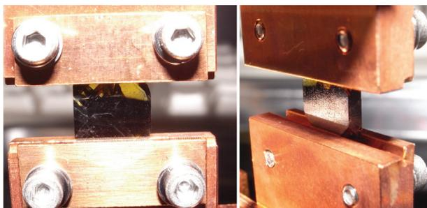
Figure 7: Photographs of the target crystal after the experiment, in which the crystal was irradiated with the 100-MeV electron beam from the linac.
