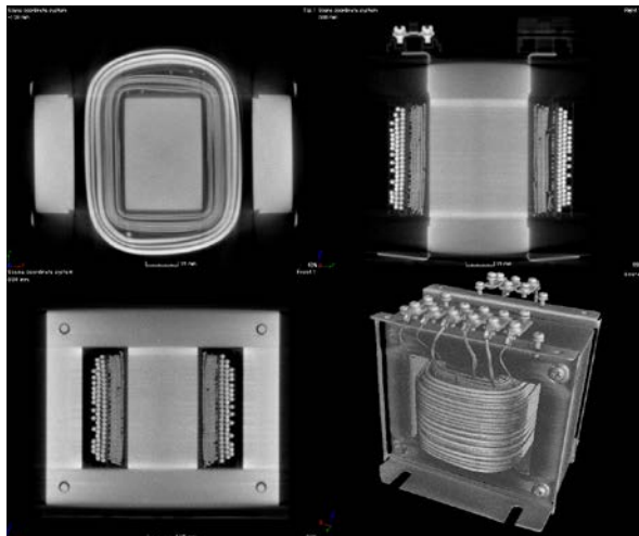
Figure 6: CT images and 3D model of the transformer.
