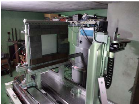
Figure 5: CT system image consists of 100 kg rotation stage and Perkin Elma flat panel with 40 cm square view.
