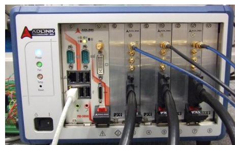
Figure 5: A setup of beam test with 48ch of multi-ch-digitizer(ADLINK PXI-2022) and CPU card(PXI-3950).
