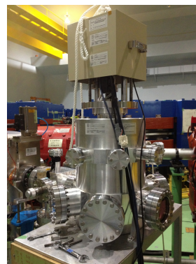
Figure 2: The irradiation port connected to the 150 MeV proton beam line. It has cryogenics and a traction control machine inside which realize measurements under irradiation of the proton beam.
