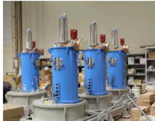
Figure 8: ACS cavities (upper) and 972MHz klystrons (lower) waiting for the installation.
