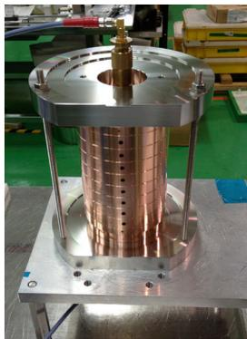
Figure 4: Measurement layout of dispersion curve of the model cavity.
