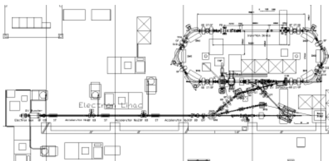
Figure 1 Electron accelerator facility at ICR, Kyoto University
